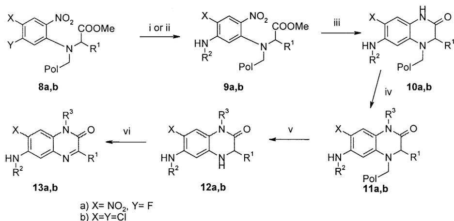
Scheme 2. Extending the diversity of quinoxalinones. Reagents: (i) amine, DMF, rt, overnight; (ii) amine, DMSO, 75°C, overnight; (iii) SnCl<sub>2</sub>·2H<sub>2</sub>O, NMP, rt, 2 h; (iv) alkyl halide, BEMP, DMF, rt, 2 h; (v) TFA or gaseous HF or HCl, rt, 2 h; (vi) air oxidation, MeOH, rt, overnight
